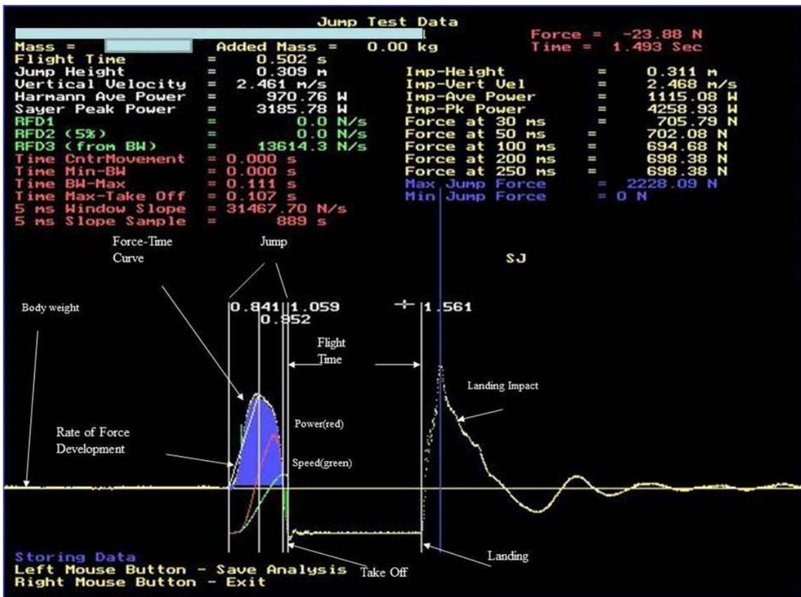
Figure 1. Force-time curve example of a static jump.
